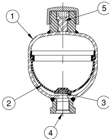
1. **Shell** - The shell is manufactured from a structural carbon steel. The non-repairable electron-beam welded construction reduces size, weight, and, ultimately, initial cost.
